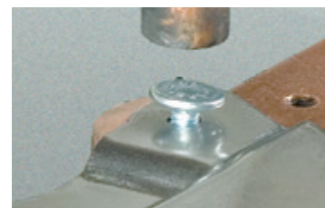
Perfect stud and sheet centring with a sleeve made of VOLCERA
