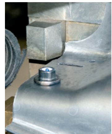
sheet and projection weld nut for an
